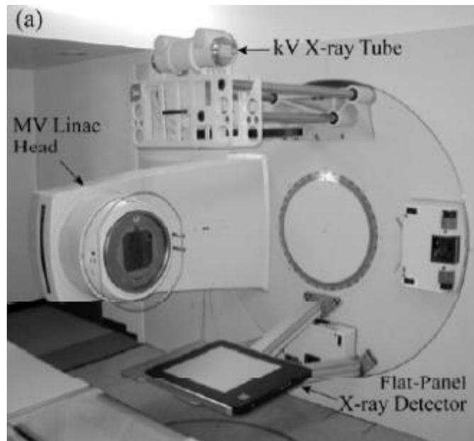
Figure 4(a) depicts a “[f]lat-panel cone-beam CT on a medical linear accelerator.” Ex. 1003, 805. The device includes a rotatable gantry, a megavoltage (MV) radiation source, and a flat panel imager opposite a kilovoltage (kV) X-ray tube. *Id.* at 804, 805.
